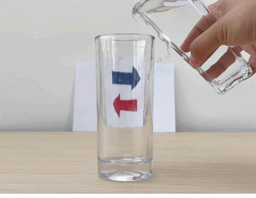
**The Science Behind It:** When light travels from one medium (like air) into another medium with a different density (like water), it changes direction. This is called light refraction. In this experiment, when water is poured into the glass, it alters the path of light rays, causing the arrows to appear "reversed". The water acts as a lens, bending the light and creating this optical illusion.
