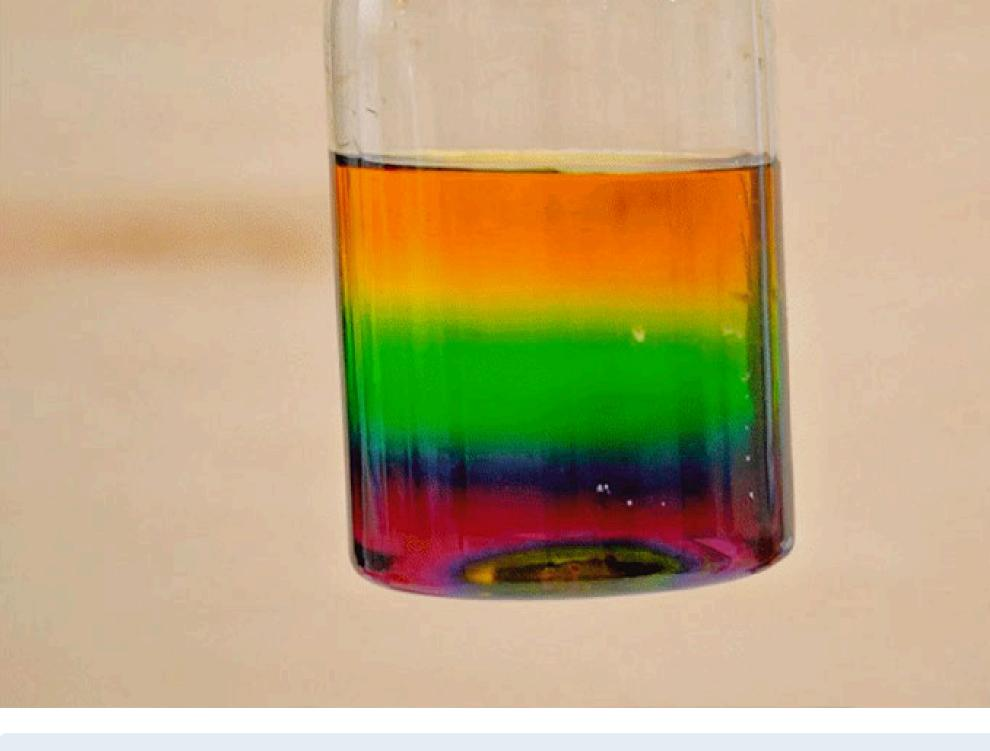
**The Science Behind It:** The density of a liquid determines its weight. Water with more salt is heavier and sinks to the bottom, while water with less salt is lighter and floats on top. When you carefully pour in coloured salt water of different densities, they don't mix
